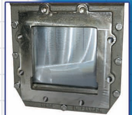
Beveled edged square gate, fully closed position, shows cavity free opening at bottom, preventing plugging
